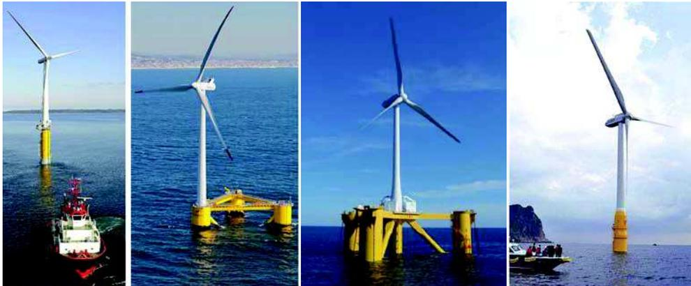
Figure 5. Prototypes of floating wind turbines (from left: a) Hywind (Statoil, 2014); b) WindFloat (PrinciplePower, 2014); c) Fukushima semi-submersible (FOWC, 2013); d) GOTO spar (GOTO-FOWT-Website, 2014)).
